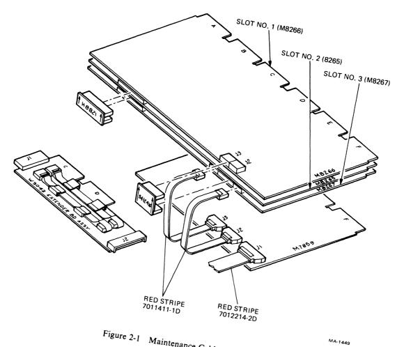
Figure 2-1 Maintenance Cable Installation
