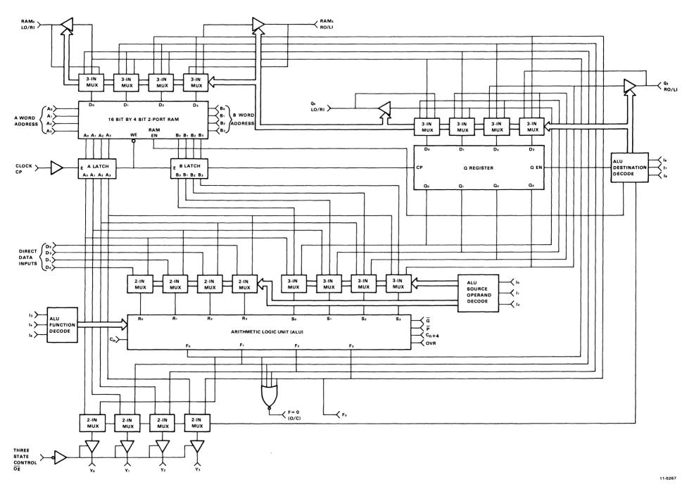
Figure 6-3 Microprocessor (AM2901)
