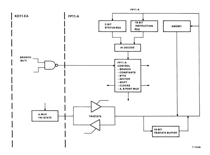
Figure 6-2 Simplified FP11-A Block Diagram
