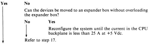
Reconfigure within the box until the CPU backplane current drain at +5 Vdc is less than 25 A.
