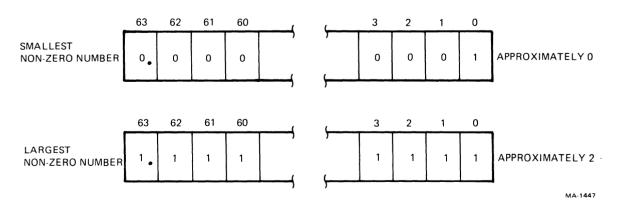
Figure 4-5 Unnormalized Floating-Point Fraction
