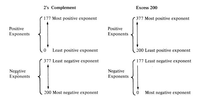
Note that an exponent in excess 200 notation is obtained by simply adding 200 to the exponent in 2's complement notation. Thus, 8-bit exponents in excess 200 notation range from 0 to 377 (or from -200 to +177). A number with an exponent of -200 is treated by the FP11-A as 0.
