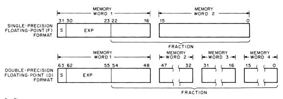
$S=Sign \\ EXP=Exponent in excess 200 notation (refer to paragraph 3.3.1.2.), Fraction = 23 or 55 bit fraction in sign and magnitude format.$
