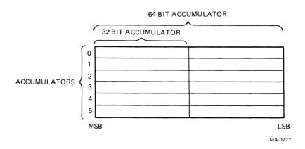
Figure 5-1 Floating-Point Accumulators
